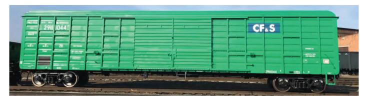
The boxcar model 11-2135-01 is a 4-axle covered boxcar with widened doorways and increased body volume (without internal body sheathing). The model is designed to ensure the safety of cargo in adverse weather conditions, protection against theft and mechanical damage.
